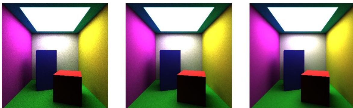
Figure 7: the cornell box rendered with our path tracer. From left to right: 2048 samples/pixel, 4096 samples/pixel, 8192 samples/pixel. As the amount of samples increase, the noise becomes less noticeable.
